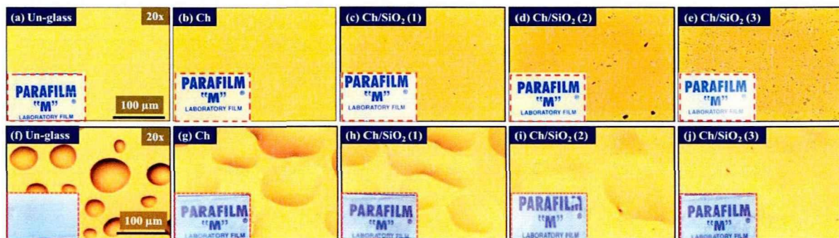
Fig. 5. 7. Optical microscopy and photograph pictures of composite chitosan coating layers (a, b, c, d, e) after coating (f, g, h, I, j) after the antifogging cold test. The photographic pictures in the optical images were taken after each test.
