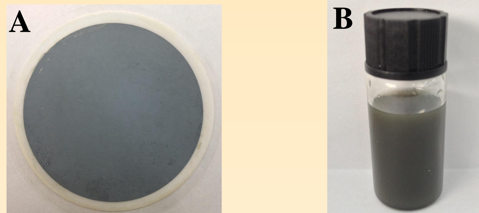
Fig. 3. (A) Exfoliated MoS 2 on the filter paper substrate; (B) The supernatant after sonication of MoS 2 in the solvent NMP.
