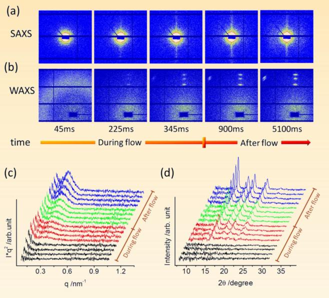
At 130 °C, SAXS images show streak scattering and WAXS images show the monoclinic  $\alpha$  -form crystals with a high degree of Surprisingly, orientation. stacks of lamellae were observed during flow, as demonstrated the by of scattering appearance maximum.
