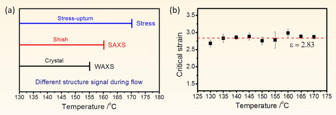
Unexpectedly, the critical true strain for nucleation remains almost constant around 2.83. Evidently, the above experimental results demonstrate that ERM for FIC is not valid under strong flow.
