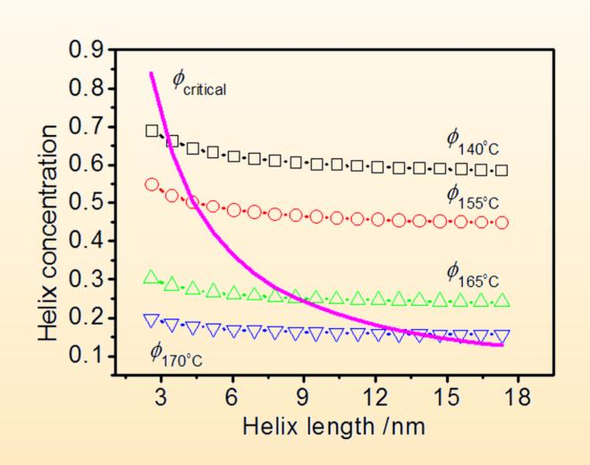
nucleation is sufficient to both the generate concentration and compatible alignment of helixes. Coupling between coil-helix and orientational transition ordering drives packs of ordered helix sequences into shish bundles, which further transform into normal crystal.
