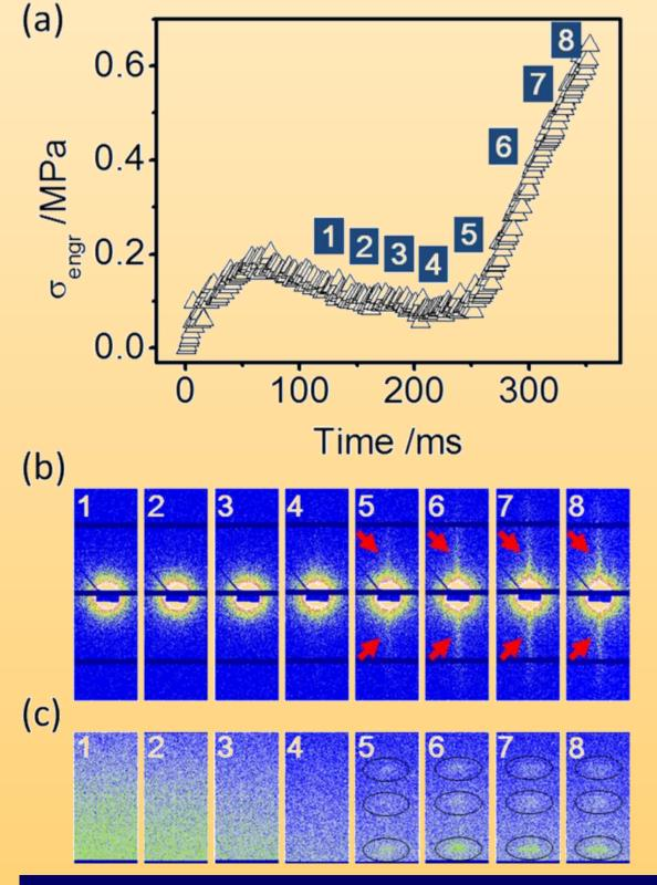
At 140 °C, the onset time for stress-upturn is about 234 ms, which corresponds to a strain of 2.84. The onset strain of stressupturn is accompanied with the formation of crystalline shish, as evidenced by the simultaneous appearance of the streak signal in SAXS images and the 2D concomitant highly orientated diffraction of monoclinic  $\alpha$ form crystals by WAXS. Here we define the onset strain of SAXS streaks or stress-upturn as the critical strain for nucleation.
